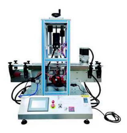
This machine includes automatically cap sorting, cap feeding, and capping function. The bottles are entering in line, and then continuous capping, high efficiency. It's widely used in industries of cosmetic, food, beverage, medicine, biotechnology, health care, personal care chemical and etc. it's suitable for all kinds of bottles with screw caps.
