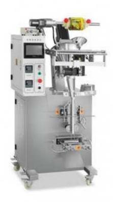
DS100P can automatically finish counting the quantity of bags, filling, sealing, cutting, with packaging material polytene, BOPP film, and tea filter paper. Equipped with photoelectric cells and auto constant temperature device, steeples speed governor, PLC and auto counter.
