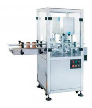
This machine is suitable for packaging various round cans, such as tin cans, aluminum cans, plastic cans, and paper cans. The machine has two pairs (four) of wheel seam seals. To seal round cans of different specifications, you only need to replace the pressure head, turntable, and lower cover device. High production capacity, wide application range, high degree of automation and easy adjustment. Suitable for canning production line equipment.
