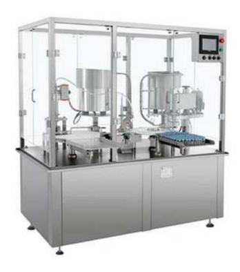
Automatic injection vial filling machine for 7-30ml vial consists of turntable, linear conveyor system, graduator, 4 head filling device, roller type stoppering servo motor driver the 4 filling auger to fill with the help of graduator position system.
