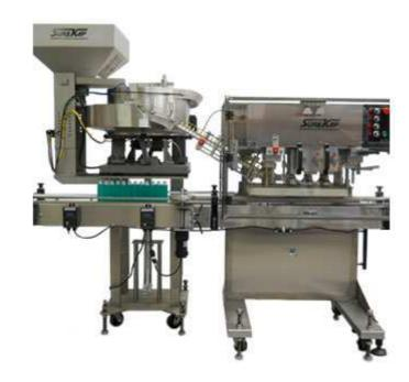
The SK6000-SP Capper is a fully automatic, straight line, six spindle capper with a head-mounted, heavy-duty straight chute. This model is designed for special and high-speed applications.
