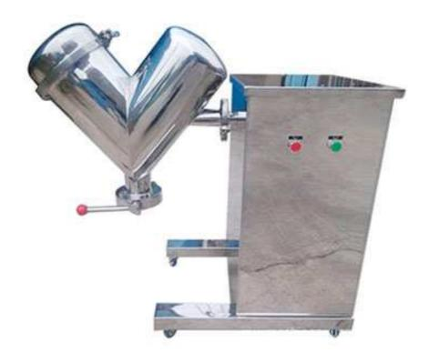
Small V Mixer Machine adopts the principle of gravity diffusion to mix, and the pressure feed to the material is small, and it will not shear and pulverize the material. The cylinder body is made of high-quality stainless steel, and the inner and outer walls are polished. There is no pollution to the material during the mixing process, low power consumption, and easy cleaning.
