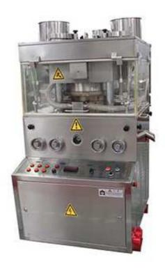
This machine is a double-press; automatic rotation and continuous tablet press for pressing granular raw materials into tablet. It is mainly used in pharmaceutical, chemical, food, electronic industry and so on.
