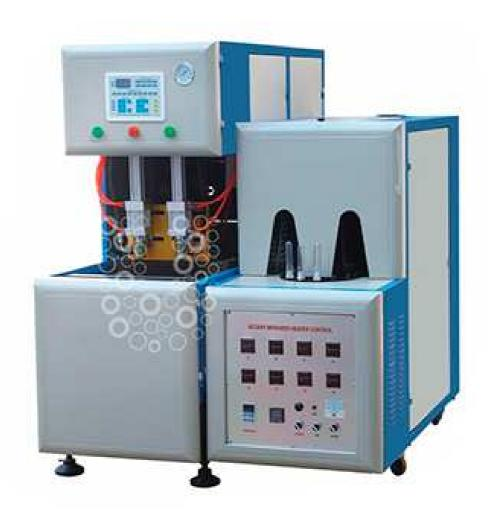
Semi-automatic blow molding machine basdesigned by CE standard. With microcomputer controlling system, it controls various technical parameter needed more accurately and more steadily. Only one person without special training operates it more easily and more safely. UT-1200 blow molding machine is fit to blow carbonated beverage bottles, mineral water bottles, cosmetics bottles and hot-filling bottles, especially oil bottles with handles.
