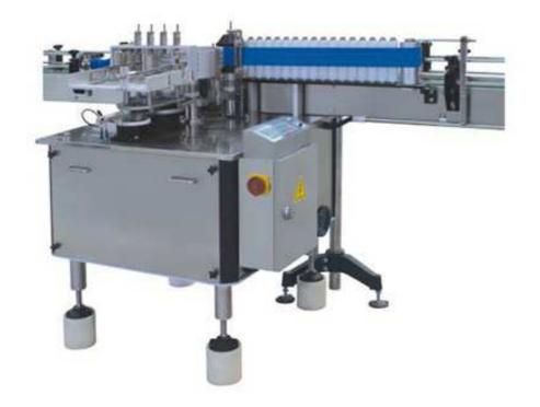
It is a pasting labeler. It takes some resin adhesive by sticking rod firstly, then some labels by labeling rod to vacuum belt and label the labels on the bottles.
