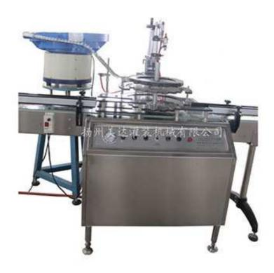
This machine consist of spay head machine, spay head presser and PLC programmed control. Sort and conveyor of spay head, self compress of spay head and aerosol cans, all can come true. It is excellence in high speed, low noise and high automation.
