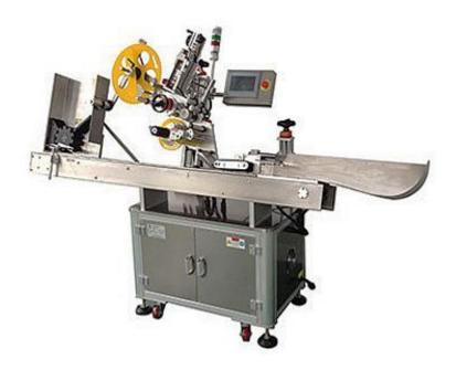
This machine is suit for small round objects which can not stand stably when labeling, such as ampoule, injection, penicillin, pen, battery, tubes and so on, machine conveyor is custom made depends on client product size.
