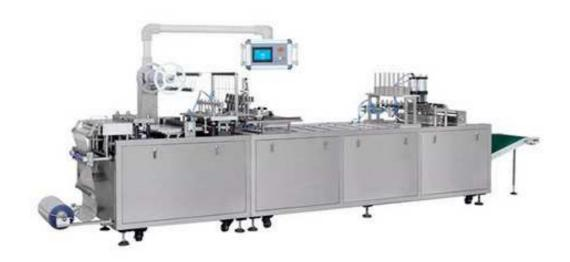
BA-600 linear pallet automatic blister card packing machine can form blisters, fill (optional), seal blisters to ready-made cards automatically. It is flexible and has high packing capacity for large runs.
