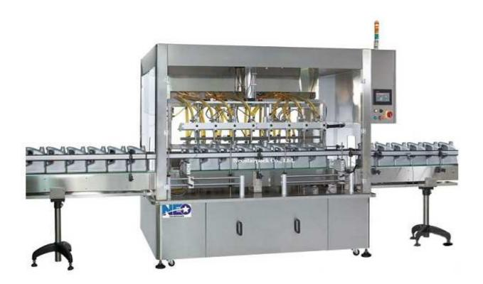
FG-585S High speed lubricant filler is suitable for lubricant oil filling requirement with massive filling volume from 1 liter to 5 liter. Controlled by servo motor make filling precise and each nozzle can be adjusted individually.
