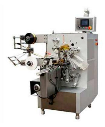
This machine is designed in 2 versions, single twist wrapping version and double twist wrapping version, to meet different requirement from customers. Perfectly works with multiple types of chocolate, like cone type, rectangle type, round type etc.
