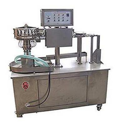
The automatic ice or jelly lolly filling and sealing machine is designed for packaging fruit jelly, ice pop, as well as various liquids such as water, yogurt, and various different types of drinking.
