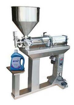
The desktop semi automatic liquid filling machine, mainly adopt the stainless steel, it have good resistant acid and alkdi, certainly it is include the good corrosion. It can meet oil, sweet chili sauce, juice, injection, shampoo, washing-up liquid and paste etc, we can adjust the speed of filling when the machine working. At the same time, the machine adopt the vacuum recovery or moment closure methods, it is stop the liquid dripped.
