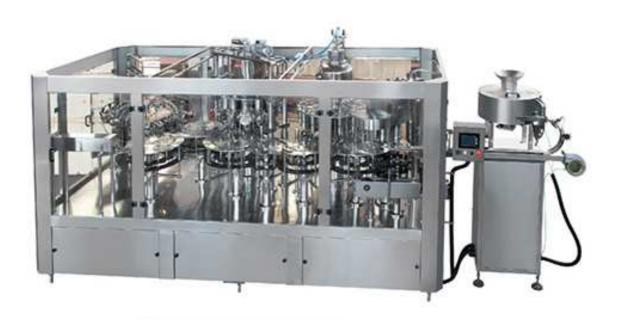
Fruit flesh hot filling equipment adopts bottle neck holding transmission technology to realize fully automatic bottle rinsing, pulp filling, and juice filling and cap screwing. It adopts single cavity plunger type of fixing filling volume technique and is equipped with perfect temperature control system, reverse-flow system, automatic cleaning system and control program. Each machine element that contacts with the liquid is made of high quality stainless steel and food-grade rubber.
