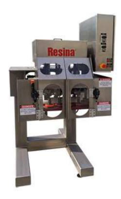
The NRT-40 in-line cap TORQing system is designed to ensure proper cap tightness when a simple capping machine or two-station retorquer is simply not enough. This retorquer finds its niche in high speed applications, or for products that must maintain precise closure tension. It comes with our NEMA 4 control panel, electronic safety interlocks, complete enclosure, and 8' of conveyor.
