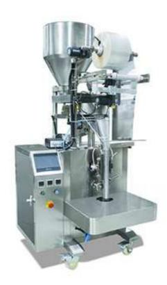
Triangle bag packing machine is suitable for packing chocolate balls, candy, chewing gum, puffed rice and so on.
