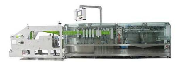
This machine is completely designed with the newest technology, and it has so many different specifications from other machines. It can work with Doypack or 3-4 side sealed pack. It can fill from 600gr to 3000gr. All of the parts made with stainless steel. In optimum conditions it can reach 160 packs per minute. It works with two filling head. For all of the electrical and pneumatic parts world-known brands used. And also this machine has half cut unit.
