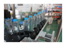
Main plate: adopts 12 station main plate and adopts cam positioning, which can accurately find the product positioning point and rotate to the labeling position, which can realize high speed positioning labeling and keep the product in the same posture.
