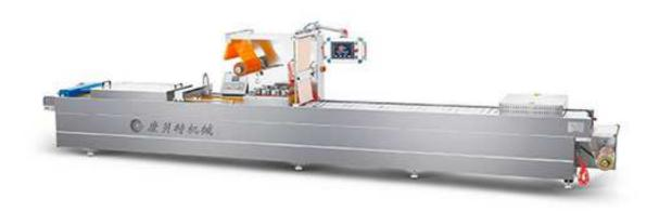
Thermoforming (from wikipedia.org) is a manufacturing process where a plastic sheet is heated to a pliable forming temperature, formed to a specific shape in a mold, and trimmed to create a usable product. The sheet, or "film" when referring to thinner gauges and certain material types, is heated in an oven to a high-enough temperature that permits it to be stretched into or onto a mold and cooled to a finished shape. Its simplified version is vacuum forming.
