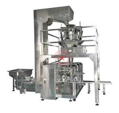
This Automatic Gusset Bag Pouch Filling Sealing Packing Machine is a low cost mini doypack packaging machine. It is for coffee beans / pods packaging fully automatically.
