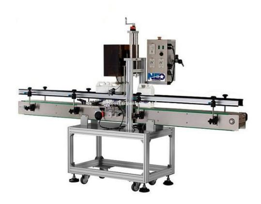
Automatic indexing spindle capper NCW-310 is the best choice for various bottles with small production. Capping height and speed are adjusted by hand wheel and speed knob easily, there is no complex parameter setting or interface. Capper will guide bottles and start capping right after caps placed by operator.
