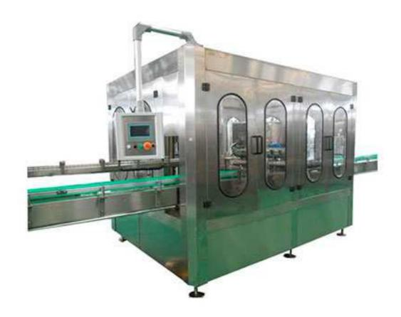
This Automatic Bottle Fruit Juice Processing Machine has washer, filler, capper three functions in one body, the whole process is automated. It is suitable for high temperature PET bottled juice and tea beverage filling. It adopts advanced micro-pressure gravity filling principle. It has a complete perfect recirculation system, and can also achieve a separate return gas without contact with the material, avoiding secondary pollution and oxygen. It is made of high quality SUS304 stainless steel.
