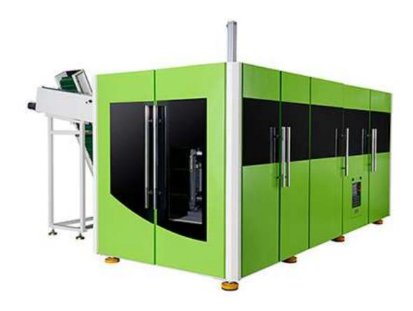
WBB-3-7 5L PET Blowing Machine is suitable for big bottles from 3L to 7L, like mineral water bottle, oil bottle and other PET bottles customer need. It is the most wanted automatic Bottle Blowing Machine for the companies who want to upgrade their production of 5L lines, to instead of semi-Automatic Blowing Machine.
