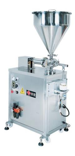
The ointment filling equipment is semi-automatic volumetric filler for high cohesion material such as gel, cream and etc.
