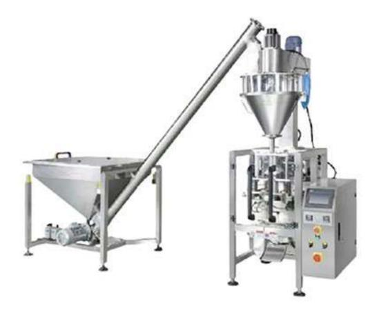
Production line powder screw packaging machine adopts intelligent microcomputer control, complete functions, simple operation, convenient maintenance, and small space occupation. The high speed powder packaging machine unit is also equipped with a touch screen operation interface. The debugging of new machines or the debugging of new materials is simple and quick, easy to use, and the powder packaging machine The material contact part is made of stainless steel.
