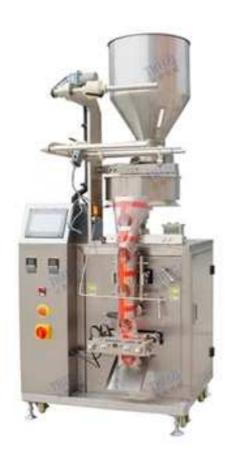
The popcorn filling machine is with function of automatic filling, film forming and making bags, sealing and cutting, date coding etc. Suit for packing dry granule item like seed, popcorn, rice and grain, salt & sugar, peanut, sachet washing powder etc.
