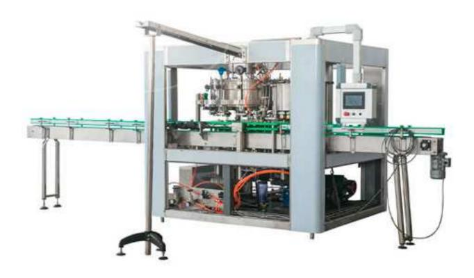
Our newly designed BCGF serious monoblack beer filling machine is designed for aluminum can and metal tin can filling, it can suit for can size between 150ml to 750ml, can customized to maximum of 1000ml. On machine surface is only leaving 3 points of bearing support point which makes drainage so easy and without any dirt stain.
