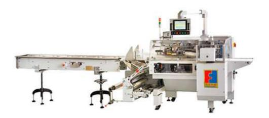
FFC-M series packing machine are specially designed for assembly packing of several blocks. Adopt box motion packing style, This machine has more sealing time has more sealing pressure. This machine adopts fi Im bottom sending to automatically wrap, form and seal, solve the problem of packing several blocks without tray, save film. Also we can design the film width 720mm or 820mm to satisfy the customer's requirement.
