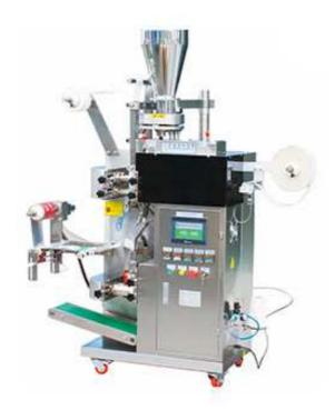
This is our economic model tea bag packing machine, it makes filter tea bag with cotton thread, tag and outer heat sealing envelop, this tea bag size can be customized, we will recommend most suitable tea bag size, and the speed 30-50 bags/min, there is date printing machine optional.
