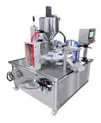
This liquid flinging machine is specially designed for making honey spoons, and molds of corresponding sizes can be customized according to customer needs.
