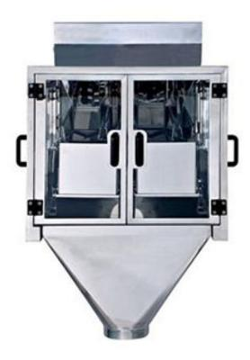
The dual head linear weigher is able to weigh 2 different items at the same time, and each head has a weighing range of 20-3000g. This linear weigher is designed to weigh tiny granules with a diameter below 20mm, like seeds, white sugar, dried fruits, washing powders, and more.
