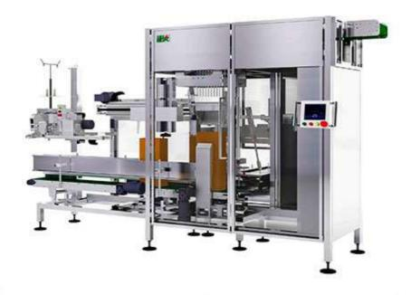
ZDQDR-160 bag packer is used for pillow bag and has the functions of auto conveying, bagging, and sealing. This machine has good bagging effect and high stability. Arrangement configuration can be customized based on customer's requirement, and has a strong adaptability to consumable materials and can use lower-cost PP bag.
