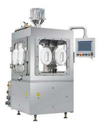
The SKF 703 platform offers all features and functionalities from the SKF 700. It offers a washable containment concept (WIP) ensuring highest protection class for operators, up to OEB 4product requirements (1.0-10.0  $\mu$ g/m<sup>3</sup>). The SKF 703 is able to produce small batches for research and development or clinical trial supplies.
