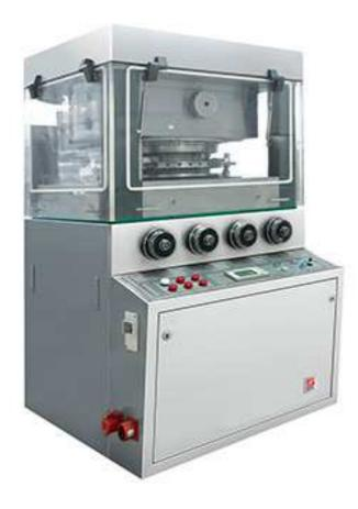
This machine is a double-press type, continuous automatic tablet press for pressing granular raw materials into tablets. It is mainly used in pharmaceutical industry and also the chemical, food, electronic industries.
