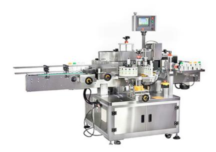
This model is suitable for the one or two side labeling, or round bottle labeling in various industries, such as shampoo, detergent, oil bottle, cosmetic care products, lotions, and sauce. The wrap around device in same unit for round bottle wrap around labeling applications. Just switch the mode for flat or round bottle for one or two labels labeling application.
