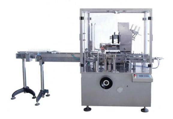
This machine is suitable for scratch, punch, soft al/al strips, wound paster, ointment plaster, facial mask, coffee bags into carton automatically. On line product feeding and detecting, leaflet fold (1-4folds) and feeding, leaflet detecting, canton opening and forming, products and leaflet pushing into carton, printing batch number, sealing carton with tuck-in or hot melt glue device. Automatically reject lacking of leaflet or product and finished product out.
