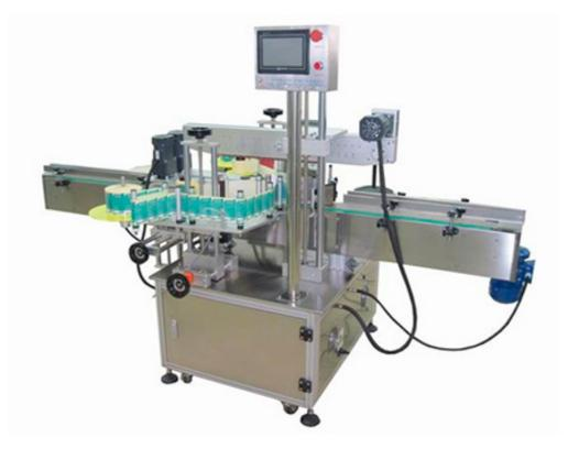
We provide double side labeling machine model SBSL-100DF for applying labels on front and back side on oval, round, hexagonal or flat bottles with output up to 100 labels per minute depending on products and label size. It is synchronized with top holding top holding belt system that ensures the straight position and maximum stability of oval shaped bottle. It is one of the most elegantly designed, versatile linear labeling machines to meet the requirements of customers.
