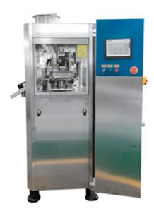
High speed Automatic Rotary Tablet Press Machine which totally meet GMP, ISO, and USA FDA requirement. The Punch Type (EU) is D/B/BB/BBS for customer to choice.
