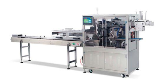
The automatic pouch filling machine is automatically feeding the bag, filling and packaging the goods. Generally used in bakeries, but also for secondary packaging or group packaging. The speed of automatic bagging equipment is about 50-60 bags per minute.
