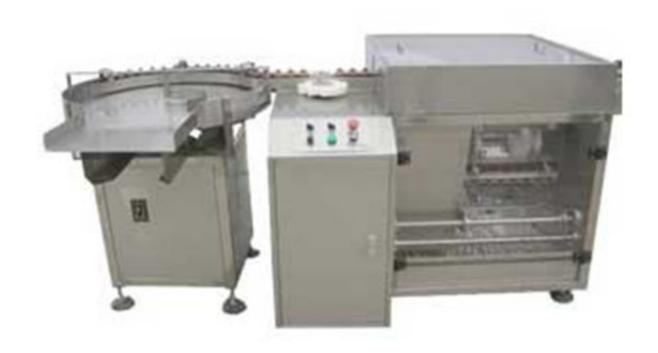
DUW Ultrasonic Bottle Washing Machine is suitable for washing 2-500ml round bottles or irregular bottles. It is used in pharmaceutical, food industrial. DUW Ultrasonic Bottle Washing Machine adopts two kinds of water and once air or three kinds of water and once air to wash the bottles. It can clean the inside and outside of the bottle and compressed air blowing it to dry. It can meet the mass production.
