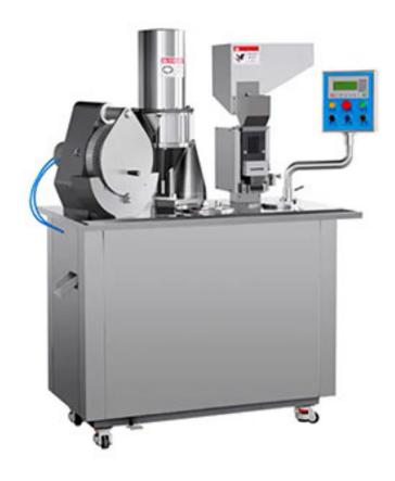
Suitable for filling #000-#5 capsules A-E type; It can fill different kinds of materials such as powder, granules, pellets, pills, etc; PLC control, filling dosage accurate is over than 97%. The touch panel can be changed to touch screen for free. Easy to operate, mold change time no more than 15 minutes.
