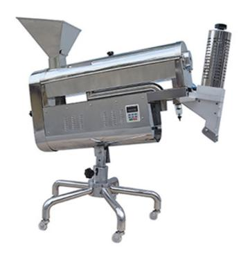
The Model JFP-110A capsule polisher with the function of sorter as well. It plays the function of not only the polishing for capsule but eliminating static electricity. It can also automatically reject low weight capsule; loose piece and fragments of capsules. It is suitable for all sizes of capsules without the need to change parts Sorter.
