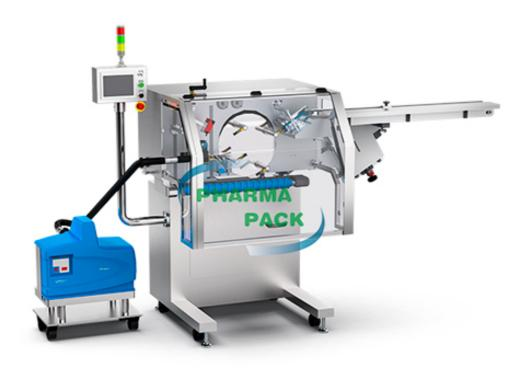
The function of LFOS-20 Leaflet inserter is: pre-folded booklets, which are manually placed on conveyor, are sucked by vacuum sucker on rotary axis are transferred forward. When bottle is coming, the sensor send signal to PLC and PLC instructs the glue dispenser to spray glue. Then the vacuum sucker press booklet on the cap and the booklet sticking process is finished.
