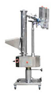
The JFP-60 vertical capsule polisher and sorter comes with the function of polishing, loading, and sorting. The inlet of the pharmaceutical machinery can be connected with the outlet of various kinds of capsule filling machine. In addition, the outlet of the product is capable of working together with metal detector, realizing joint production.
