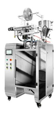
The liquid (paste) filling system is a high-precision gear pump quantitative filling device refined by CNC SUS316L stainless steel material, which has high precision, strong versatility, and is suitable for high-viscosity (pet food) materials. It is equipped with a general cleaning device as standard, but it can also be combined with a CIP cleaning system.
