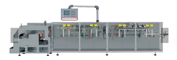
BHD-180SC is specially designed for standard spout stand-up pouches, with a maximum packaging capacity of 1000ml and a speed of up to 60 bags per minute. Hanging holes, special-shaped functions, etc. can be added according to customer needs. It is often used for packaging jelly, laundry detergent, Juice, milk and other liquids or viscosity.
