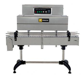
BSS series label shrink machinery are mainly used to shrink label of product in bottle shape, can shape or barrel shape with glass bottle, plastic bottle or paper cup.
